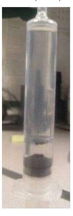
The Water and the Ethanol have mixed, separated and settled to the base while the pure Gasoline sits on top. We now have a mix of 98% Ethanol and 2% Water in direct contact with the fuel bladder and components which will begin to attack Rubber, Aluminium and Polyester [foam], the materials most used in Motorsport fuel systems.
